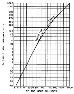
Figure 5-1. Typical voltage-transfer characteristic of the Type 1025-P1 Detector Probe.
