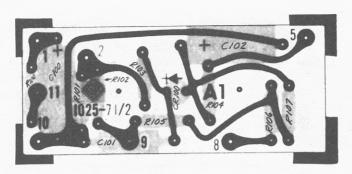
Figure 6-5. Etched-board layout for metering circuit (A1) of the Type 1025-A.
