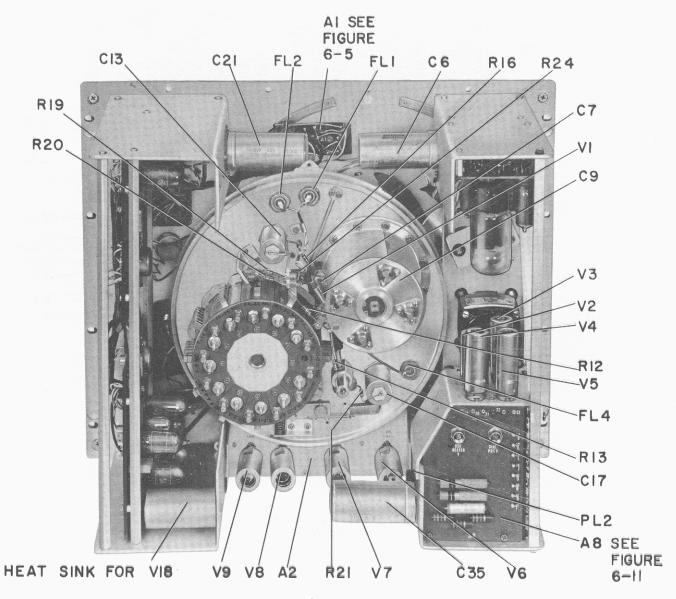
Figure 6-1. Rear interior view of the Type 1025-A.
