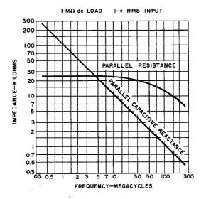
Figure 5-2. Typical input impedance vs frequency for the Type 1025-P1 Detector Probe.
