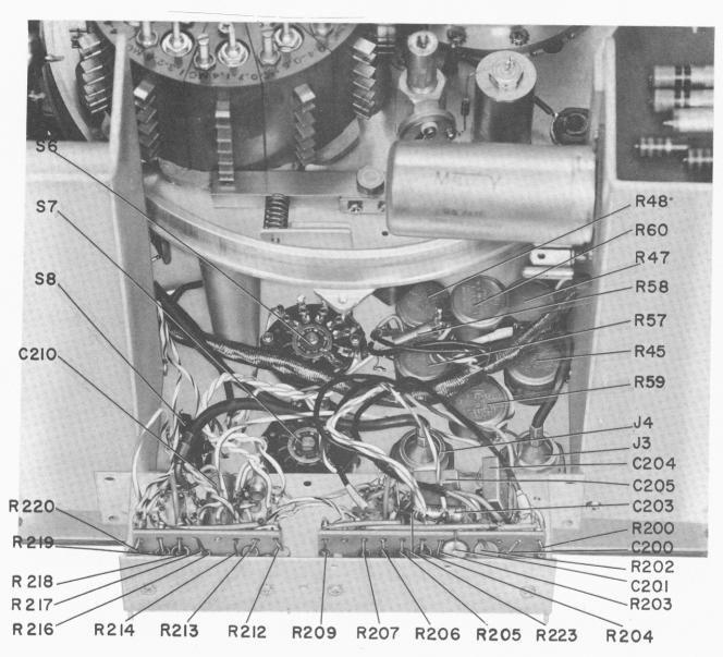
Figure 6-4. Display-output assembly (A2) of the Type 1025 demounted and folded out on its flexible connecting leads.
