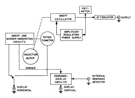
Figure 1-2. Block diagram of the Standard Sweep-Frequency Generator.
