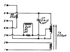
Figure 6-12. Schematic diagram of frequency-turret sectors for the following ranges:
