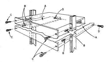
Figure 3-1. Installation of relay-rack model, Type 1025-AR.
