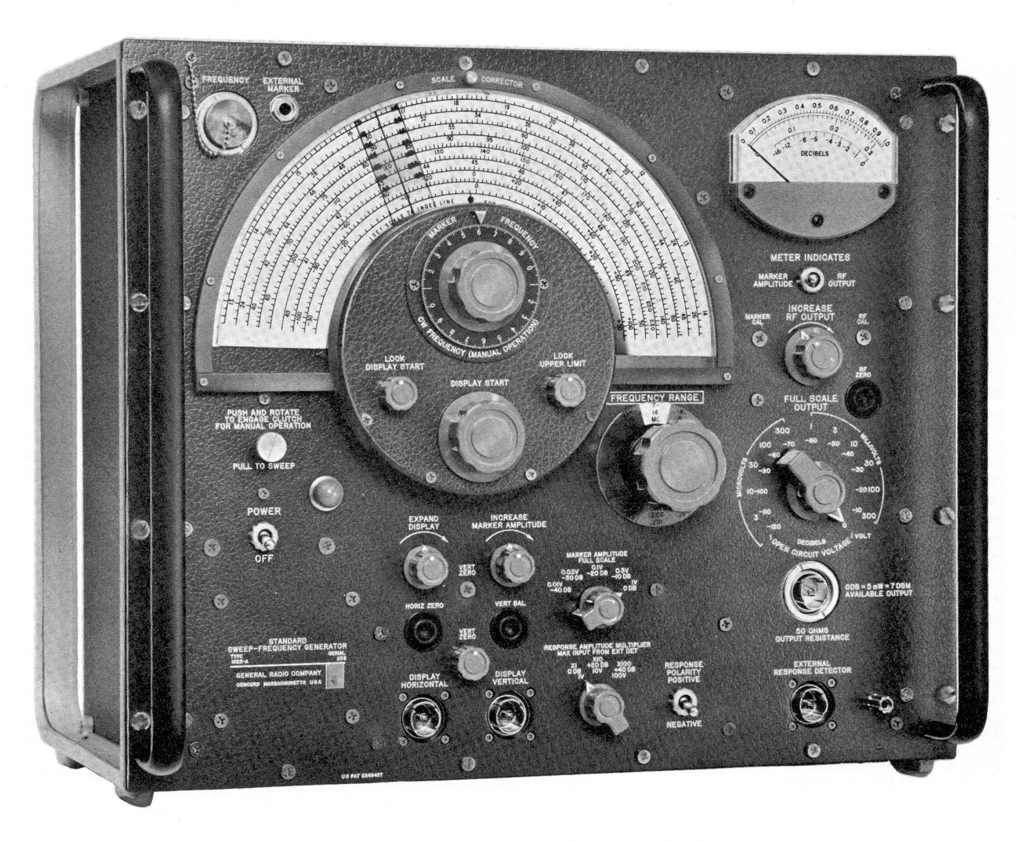
Figure 1-1. Panel view of the Type 1025-A Standard Sweep-Frequency Generator.
