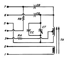
Figure 6-15. Schematic diagram of the frequency-turret sectors for the following ranges:
