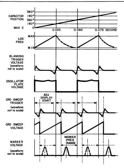
Figure 2-2. Timing diagram for one complete cycle of the Type 1025-A.
