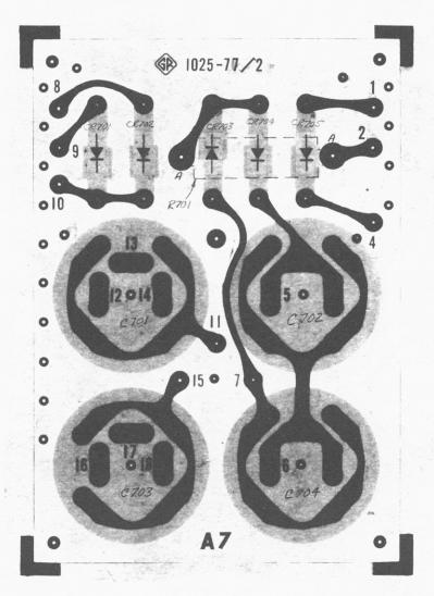
Figure 6-10. Etched-board layout for power supply (A7) in the Type 1025-A.
