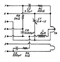
Figure 6-14. Schematic diagram of the frequency-turret sector for the 100-to-230 Mc range.
